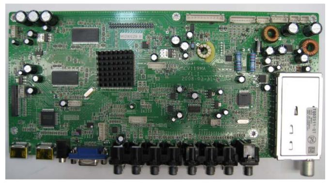
MM/311/RP Suits Panel Type: - AUO T315HW02\_V0 [Refer to C/N for Identification]
