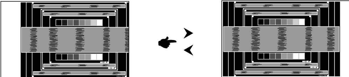
2) Stretch the right side of the picture frame to the right edge of the display area by adjusting the Clock.
