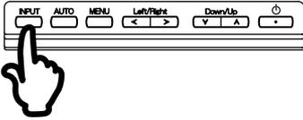
This is switched when you successively press the Input Button on the monitor or AUDIO/VIDEO/PC Button on the Remote Control as follows:
