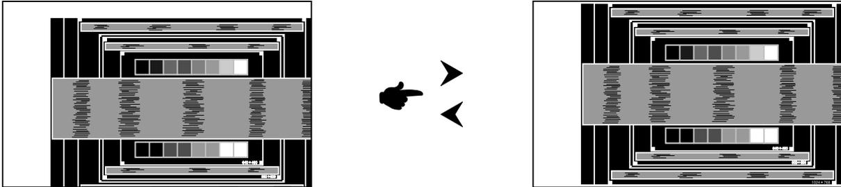
⑥ 1) Adjust the H Position so that the left side of the picture frame will move to the left edge of the display area.
