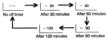
Just one minute before switching off the TV, " - 01" and channel number will be displayed on the screen.
