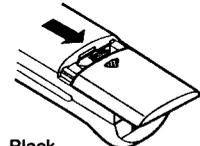
2. Plug the battery cord into the connector inside the compartment.
