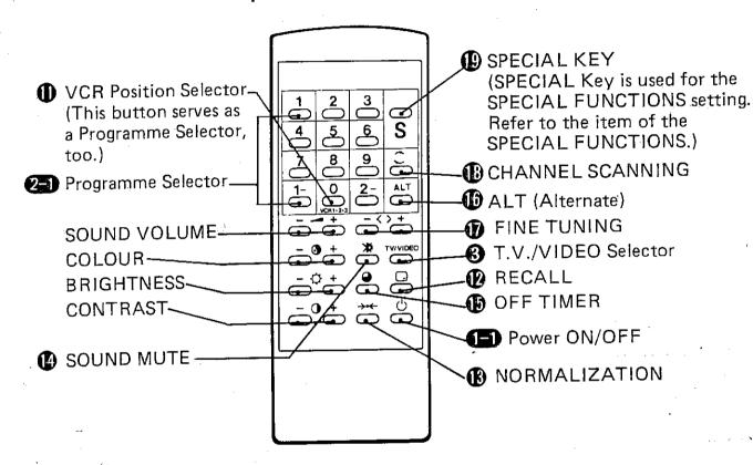
Main ON/OFF switch of the TV set must be in "ON" position before remote control operation is possible.
