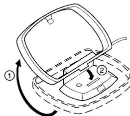
Unwind the aerial wires, then connect them to the AM LOOP ANT. terminals. Place the loop aerial in a position which yields the best AM reception, or attach it to a wall or other surface as shown in figure.
