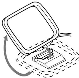
Unwind the aerial wires, then connect them to the AM LOOP terminals. Place the loop aerial in a position which yields the best AM reception, or attach it to a wall or other surface as shown in figure.
