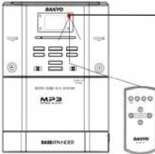
The remote control should be within approx. 7 meters at straight line to the REMOTE Sensor.
