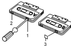
**Note:** A cassette with the erase guard tabs removed cannot be erased or used for recording and the RECORD button cannot be pressed. To record on a cassette from which the cab has been removed, simply attach adhesive tape over the tab opening.(3)
