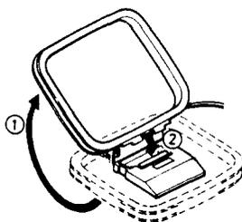
Unwind the aerial wires (about 3 turns), then connect them to the AM LOOP ANT. terminals. Place the loop aerial in a position which yields the best AM reception, or attach it to a wall or other surface as shown in figure.
