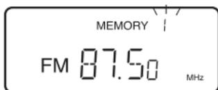
3. Within 5 seconds press the PRESET + or PRESET - button to select the channel number to be preset.
