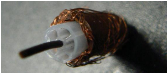
Fig. 3 75Ω 'air-cored' coaxial cable as used throughout Australia for TV antenna installations. The use of such cables must be avoided in DTV installations as they provide very poor immunity against impulse noise pickup.
