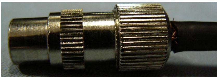
Fig. 4a & 4b 'Belling & Lee' type connectors should be avoided in DTV installations. Over time they lose their connectivity properties due to moisture ingress that tarnish the copper cable.
