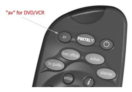
The Video and Audio signals are connected to the DVDR/VCR AV input. To record the FOXTEL/AUSTAR program, the DVDR/VCR has to be switched to this input. On our DVDRs the "INPUT" button can be used for this.
