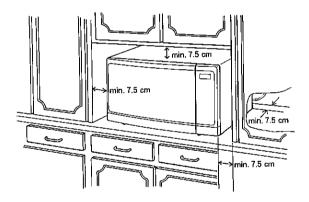
A minimum clearance of 7.5 cm is required between the oven and any adjacent walls including the back wall.
