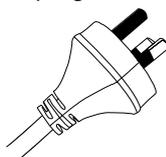
This appliance must be grounded. In the event of an electrical short circuit, grounding reduces the risk of electric shock by providing an escape wire for the electric current. This appliance is equipped with a cord having grounding wire with a grounding plug. The plug must be plugged into an outlet that is properly installed and grounded.
