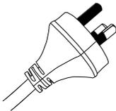
This appliance must be grounded. In the event of an electrical short circuit, grounding reduces the risk of electric shock by providing an escape wire for the electric current. This appliance is equipped with a cord having grounding
