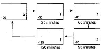
With the off timer being set and the channel display reset, the remaining time is displayed by pressing the off timer button again.
